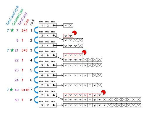
For clarity, we split the cost of each operation into the array writing part (which is identical to what we saw earlier) and the allocation part. On this short run, we see that the total cost of the most expensive operations divided by the operation number is 7. This is is the amortized number of tokens we pretend each call to uba\_add costs.
