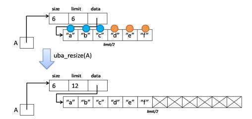
After the resize, exactly half the array is full, so our data structure invariant for tokens doesn't require us to have any tokens in reserve. This means that the data structure invariant is preserved in this case as well. In general, the number of tokens associated with an unbounded array is  $2 \times size - limit$ .
