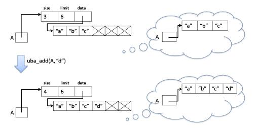
The images to the left above represent how the data structure is actually stored in memory, and the images in the thought bubbles to the right represent how the client of our array library can think about the data structure after an uba\_add operation.
