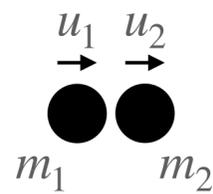
$$u_1 = \frac{m_1 v_1 + m_2 v_2}{m_1 + m_2} \quad u_2 = \frac{m_1 v_1 + m_2 v_2}{m_1 + m_2}$$
