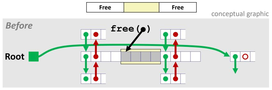
Splice out adjacent predecessor and successor blocks, coalesce all 3 blocks, and insert the new block at the root of the list
