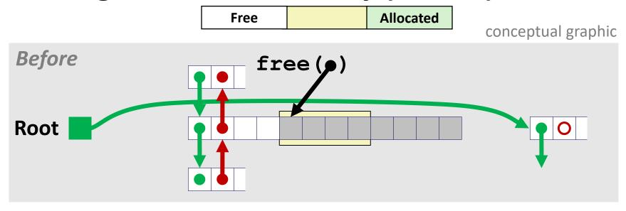
Splice out adjacent predecessor block, coalesce both memory blocks, and insert the new block at the root of the list
