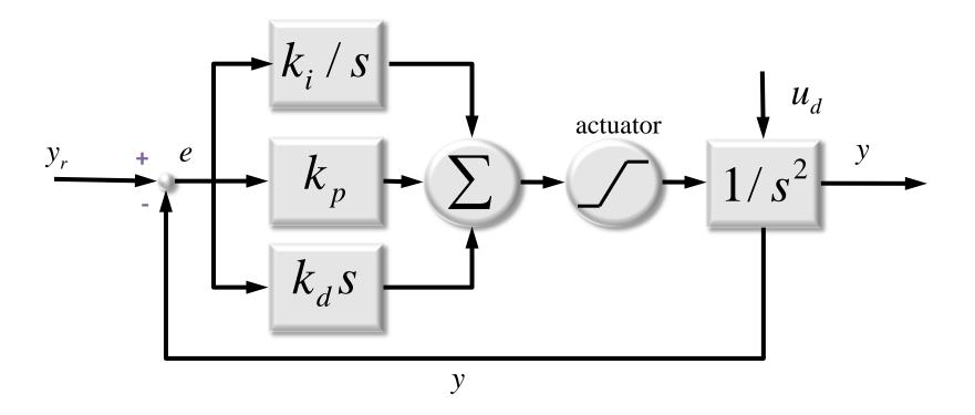
$$T(s) = \frac{H}{1+GH} = \frac{(1/s^2)(k_d s + k_p + k_i/s)}{1+(1/s^2)(k_d s + k_p + k_i/s)} = \frac{k_d s^2 + k_p s + k_i}{s^3 + k_d s^2 + k_p s + k_i}$$
