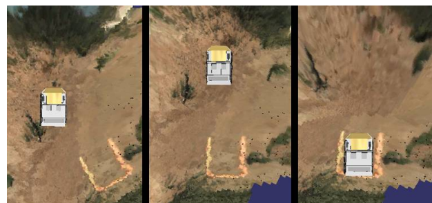
Figure 11. An overhead view allows task-specific operations, such as reversing the vehicle into a parking space without the benefit of a rear-facing sensor as shown in this sequence of three images.
