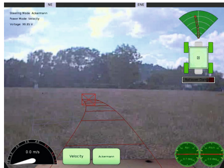
Fig. 5 Graphical User interface. A video game concept is used where annotations are overlaid with some transparency on the stabilized video.
