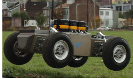
Fig. 1 Forerunner Remote Controlled Vehicle. All wheels are driven and steered. The vehicle is easily capable of 25 km./hr. speed so such ballistic motion is achievable.
