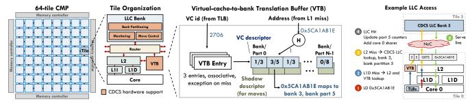
Figure 3: Target CMP (left), with tile configuration and microarchitectural additions introduced for CDCS. CDCS gangs portions of banks into virtual caches, and uses the VTB (center) to find the bank and bank partition to use on each access (right).
