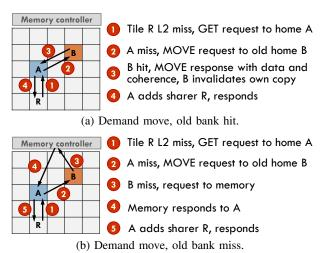
Figure 10: Messages and protocol used on incremental reconfigurations: demand moves when old bank hits or misses.
