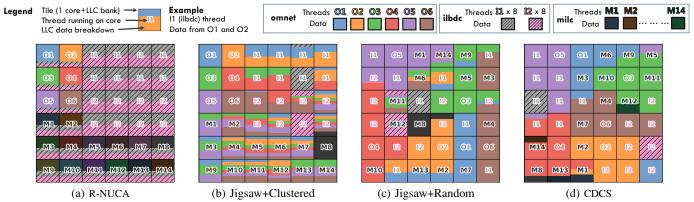
Figure 1: Case study: 36-tile CMP with a mix of single- and multi-threaded workloads (omnet×6, milc×14, 8-thread ilbdc×2) under different NUCA organizations and thread placement schemes. Threads are labeled and data is colored by process.
