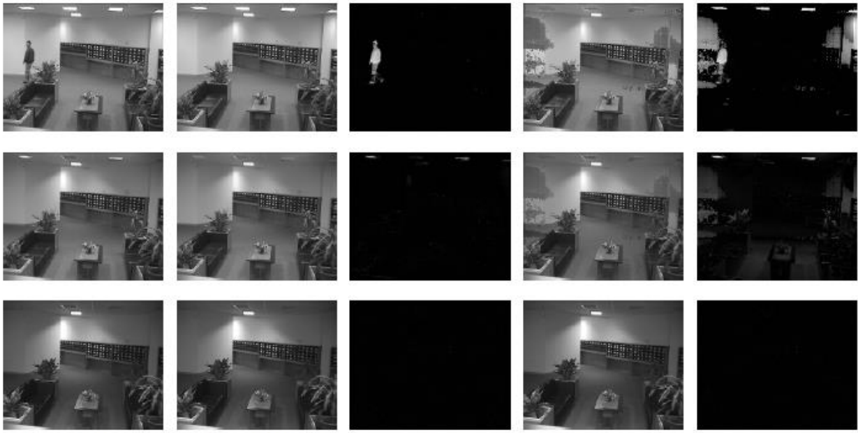
(a) Original frames (b) Low-rank \hat{L} (c) Sparse \hat{S} (d) Low-rank \hat{L} (e) Sparse \hat{S} Convex optimization (this work) Alternating minimization [47]
