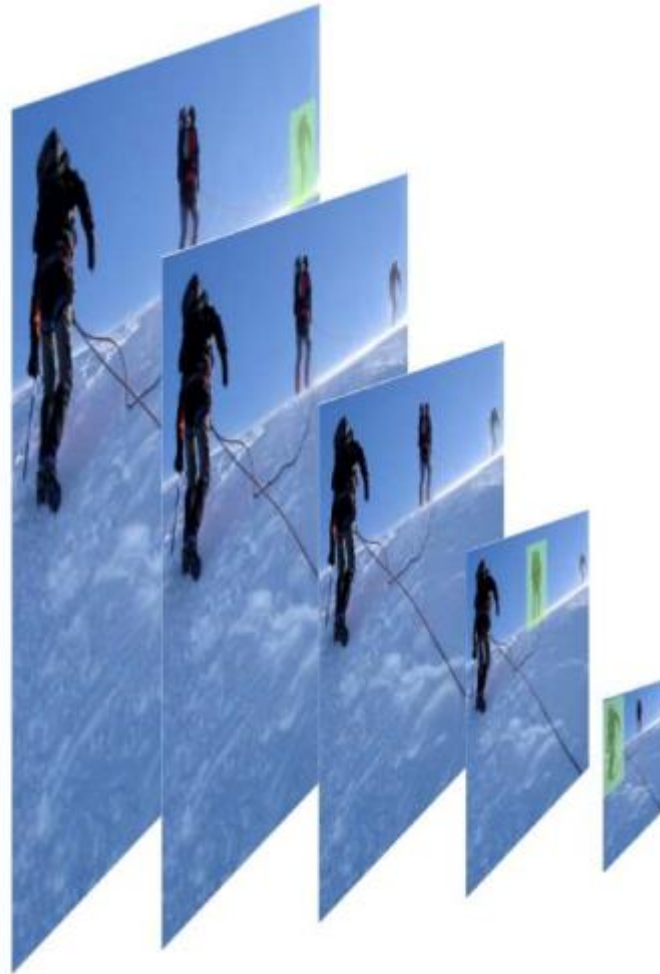
Figure 1.4: The Scale-Space Pyramid. The detector is run using the sliding windows approach over the input image at various scales. When the scale of the person matches the detector scale the classifier will (hopefully) fire yielding an accurate detection.
