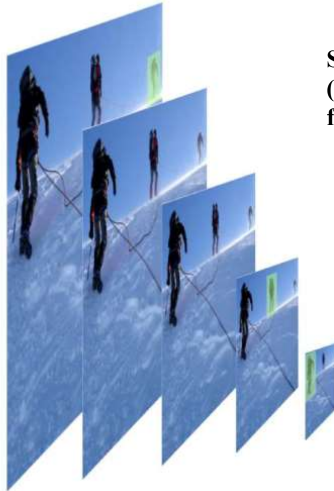
Figure 1.4: The Scale-Space Pyramid. The detector is run using the sliding windows approach over the input image at various scales. When the scale of the person matches the detector scale the classifier will (hopefully) fire yielding an accurate detection.
