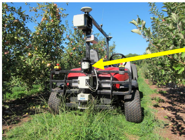
Figure 66. The APM in its new configuration. The laser range finder mounted just above the hood is the only one used for row following.
