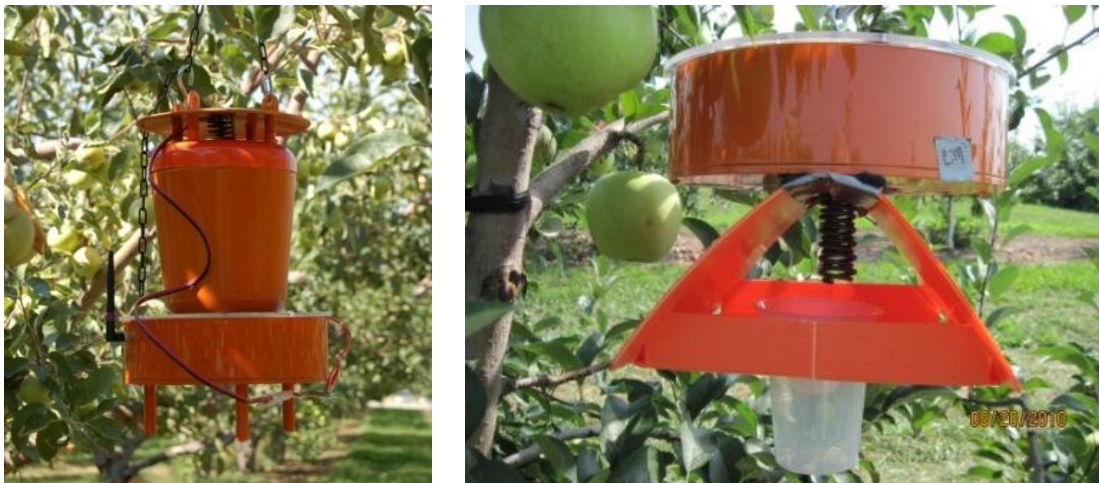
Figure 28. Modified Z-traps employing existing bucket trap (left) and delta trap (right) exterior designs.
