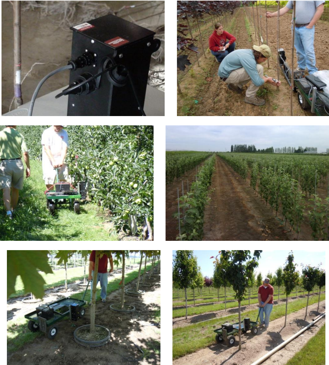
Figure 60. From top to bottom, left to right: caliper being used to determine tree diameter in a warehouse sorting operation, bareroot ornamental nursery, established orchard, bareroot fruit tree nursery and ornamental wholesale nursery in both field and pot-in-pot production systems.
