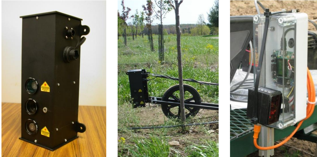
Figure 59. Second generation caliper, constant height wheel-mount and infrared sensors for counting.
