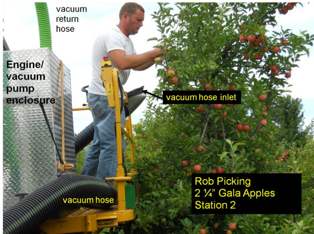
Figure 87. Close-up of DBR system showing worker and vacuum hose inlet.
