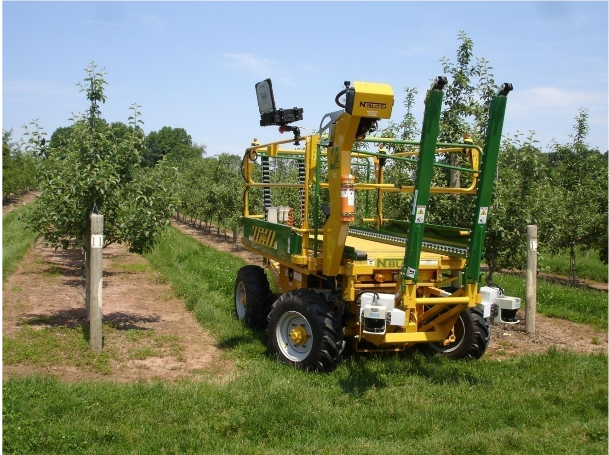
Figure 72. The automated N. Blosi platform. Two laser range finders provide a view of the world similar to the original configuration of the Toro eWorkman APM. All software, including the user interface, runs on the laptop mounted on the top rail.
