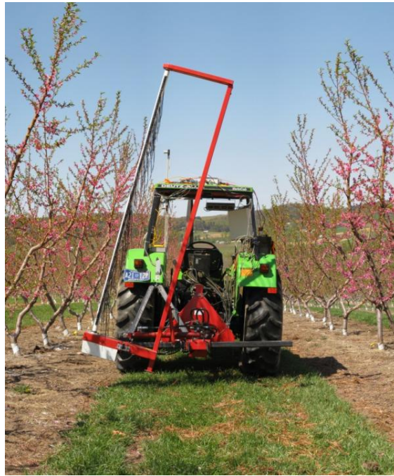
Figure 78. The modified Darwin thinner mounted onto a tractor. Note the ultrasonic mast visible above the tractor roof.
