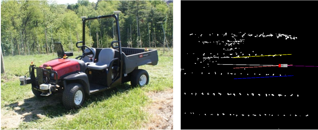
Figure 65. (Left) The Autonomous Prime Mover (APM) in its original configuration, with laser range finders mounted low on the corners of the vehicle. (Right) With the lasers at this height it was easy for sloped terrain to come into view, which presented a challenge to the row detection algorithm.
