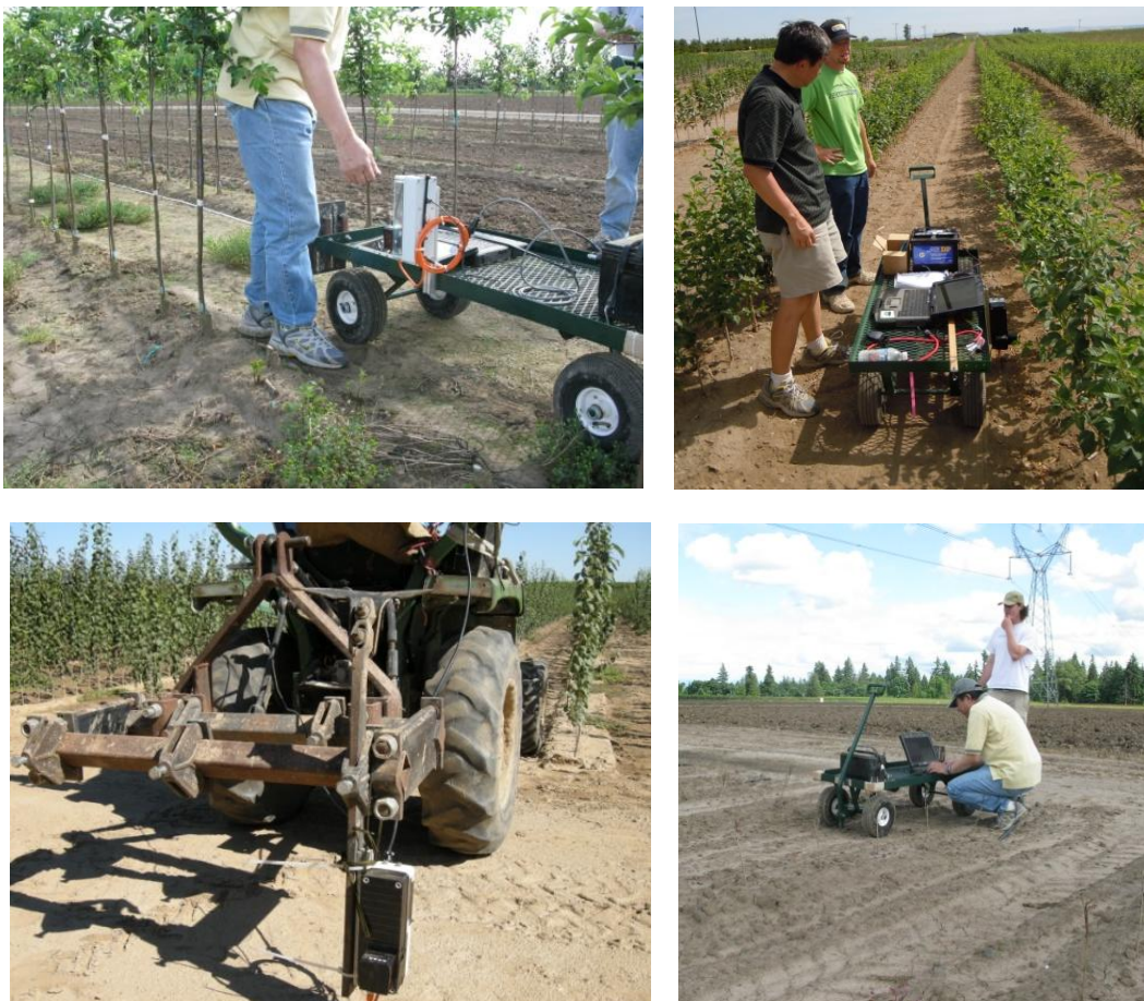
Figure 62. Infrared devices used in Year 2 to count trees in bareroot ornamental nursery, fruit tree seedling nursery, bareroot fruit tree nursery and ornamental tree seedling nursery.
