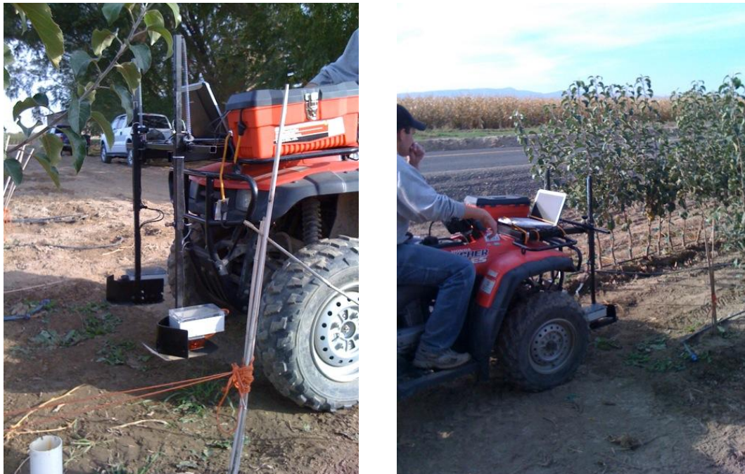
Figure 63. Crop Tech LLC utilizing CASC counter and software to count trees at a Washington tree fruit nursery.
