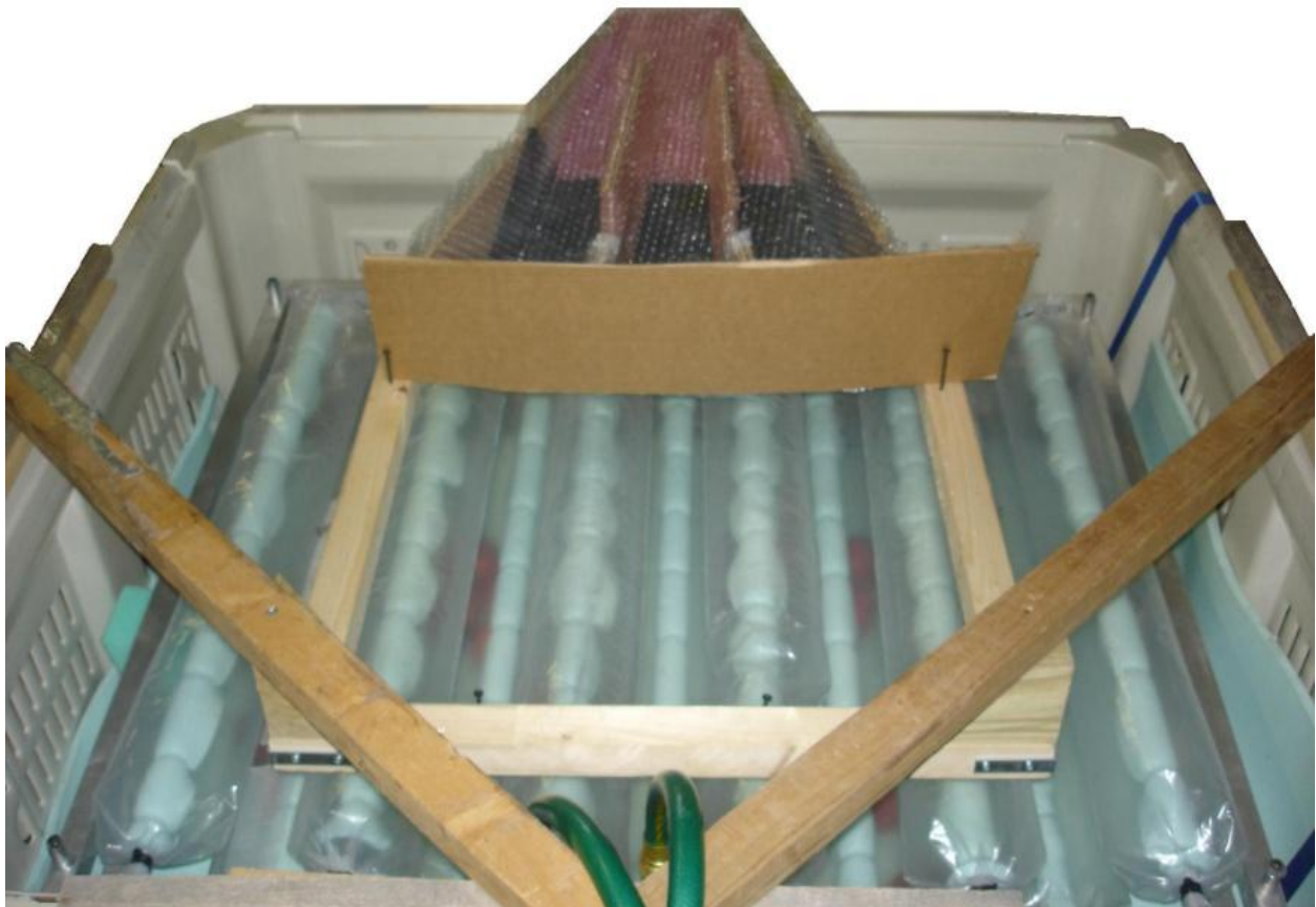
Figure 84. Pneumatic self-adjusting bin filler with test ramp.
