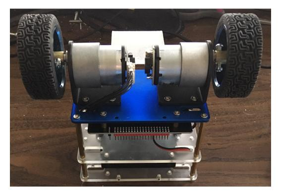
Design a feedback-only PD controller to move each wheel 1 radian. Where does the velocity signal come from? How quickly can you reach the target without saturating the motors at any point (command  $\geq 255$ )?
