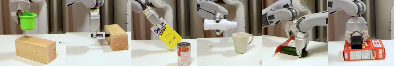
Fig. 3. The pictures show example executions of the PR2 performing the six manipulation tasks: placing, pushing, tilting, pouring, cutting, and wiping.
