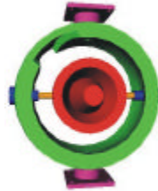
Figure 11. Partially instantiated geometry with a gimbal to couple the degrees of freedom.
