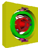
Figure 12. Complete geometry for the 2-DOF seeker.
