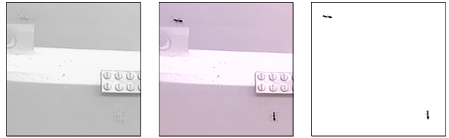
Figure 7: Use of background differencing to find moving objects. Left: Background image computed using a running locally weighted average. Center: Sample “live” image. Right: Difference between background and live image reveals the locations of two ants.
