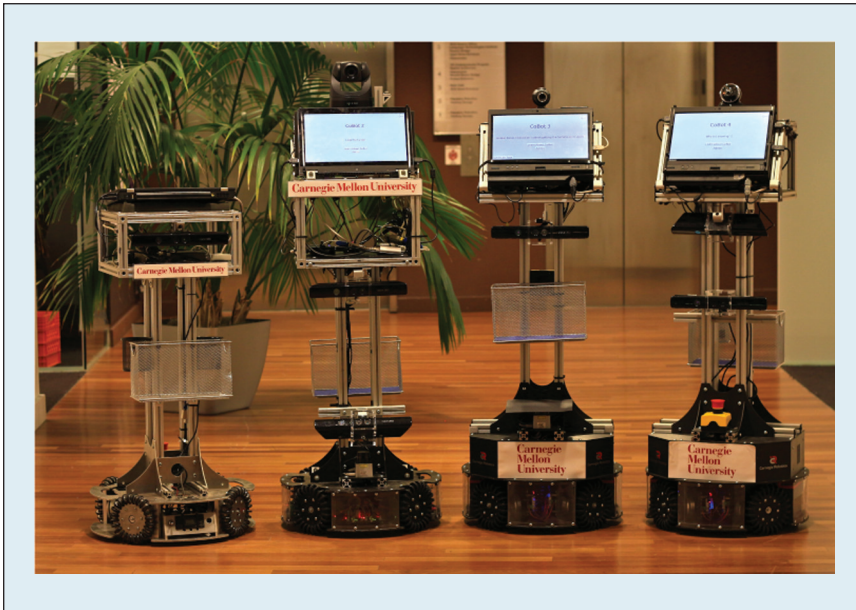
Figure 1. From left to right, CoBots 1, 2, 3, and 4, which were deployed over the course of the 1,000-km Challenge. The CoBots' sensing capabilities vary, ranging from one or more depth cameras and an optional laser rangefinder.
