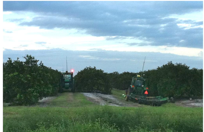
Figure 1 Autonomous tractors working in the orchard showing alternating bed rows (left) and swale rows (right)
