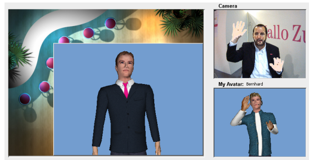
Figure 2. Example picture from user’s own camera, avatar representation generated from own camera picture (bottom right), and avatar as generated from incoming FAPs/ BAPs. Avatars are shown on neutral background.
