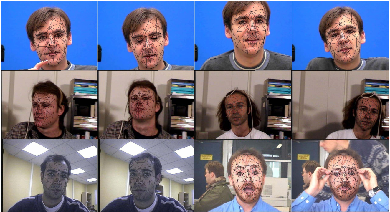
Figure 7. Frames from different video sequences showing the pose and gesture tracking. From top to bottom: Talking face video sequence, two La Cascia's video sequence and two video sequences from a webcam.
