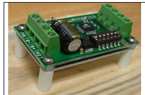
Figure 2.3: Mounted to a wood frame using standoffs
