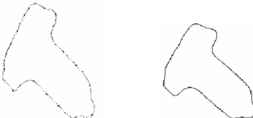
FIGURE 4.19 (a) Contour constructed for part-1 oriented at 328.51 degrees with presented approach, and (b) contour reconstructed out of compensated EFD coefficients obtained from the contour in (a).
