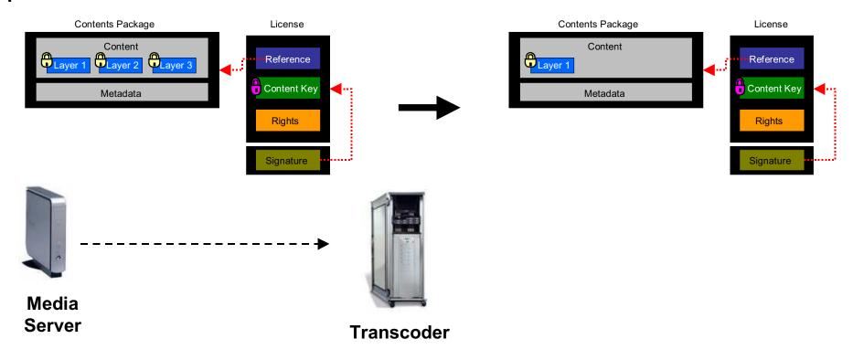
The transcoder simply truncates needless layers. It is not required that the specific compression, decoding, or encryption algorithms are implemented in the transcoder.
