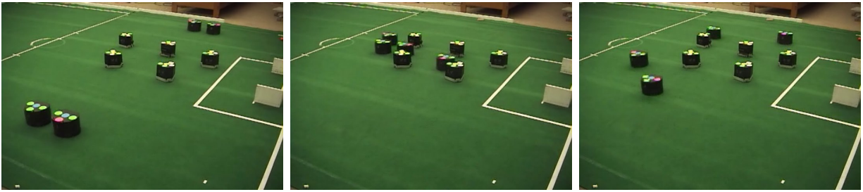
Figure 5.13: A sequence captured while running DSS with four CMDragons robots and five small static obstacles. All agents completed their 2.8m traversal within 2.8 seconds.
