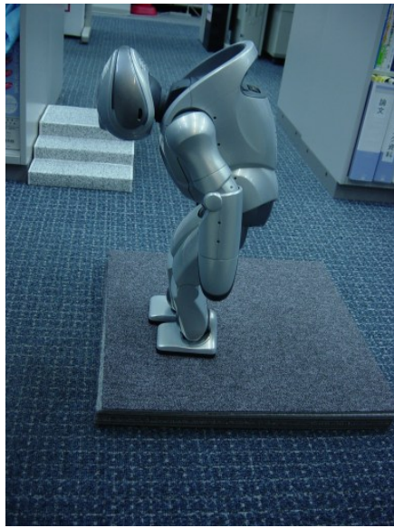
Figure 2.8: QRIO on top of an autonomously reached step obstacle.
