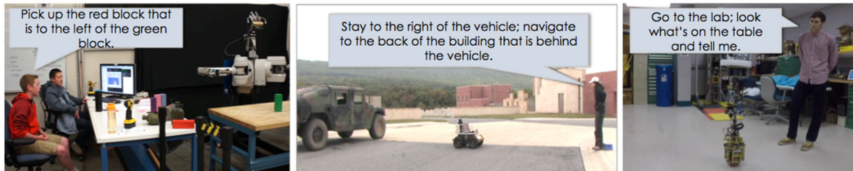
Figure 2. This figure represents natural language understanding integrated in various robot platforms: Barrett™ robot arms (left); Clearpath™ Husky robot (center); and CMU Ballbot (right; Lauwers, Kantor, & Hollis, 2005). The difficulty in integrating context-driven AI is in relation to perspective. In the image on the left, perspective is in the word 'left'. What does 'left of the green block' mean -- my left or the robot's left? In the center image, the key word is 'back'. What is the 'back of a building'? In the image on the right, there are questions as to which lab or which table and what should be told to the human.
