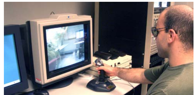
Figure 4. Initial workstation with stereoscopic telepresence capability.
