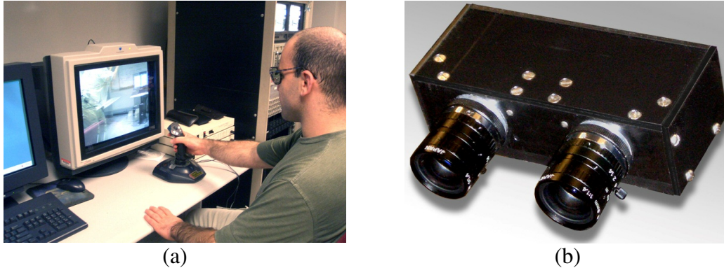
Figure 5. (a) Telepresence workstation. (b) Stereoscopic camera.
