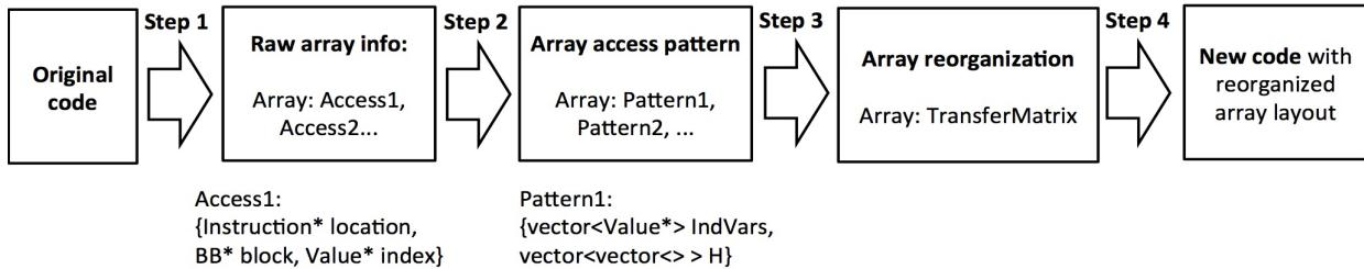
**Step 1** makes a pass on the original code to get **raw access information** for each array. For each array, we record the location (inst, block), access index variable (index), etc of each access of the array.
