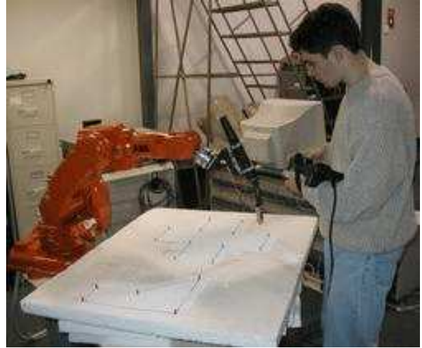
Figure 9. Creating waypoints for the patterns in Figure 8 with an ABB IRB140.
