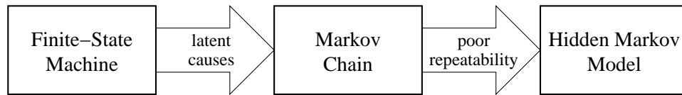
Figure 3.1: Evolution of the user model from a deterministic to a doubly stochastic system.
