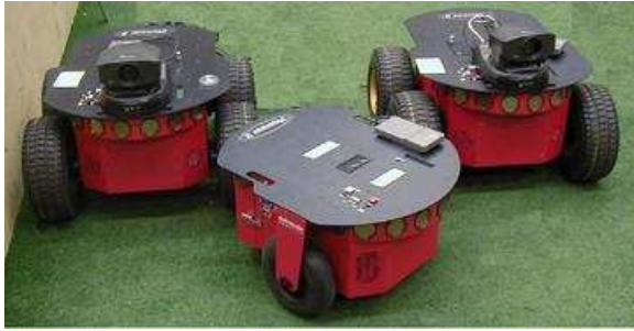
Figure 5: ActivMedia Pioneer II robots used in task decomposition: Asbestos, AgentOrange, and Saccharin.
