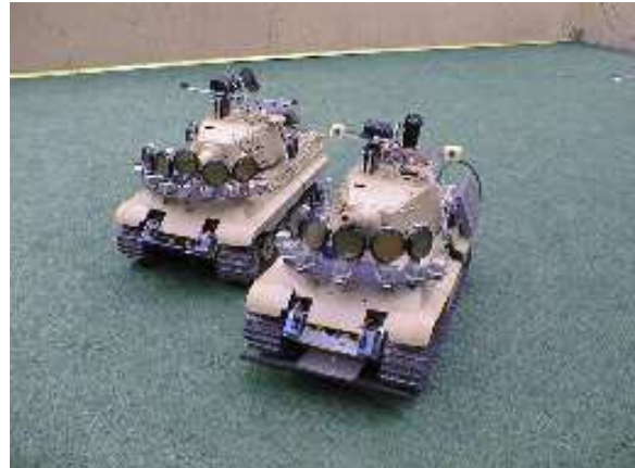
Figure 3: Robots used for mapping: Patton and Rommel.
