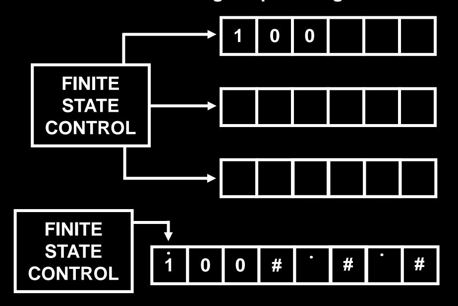
Theorem: Every Multitape Turing Machine can be transformed into a single tape Turing Machine
