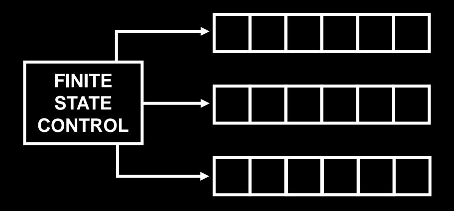
$$\delta: \mathbf{Q} \times \Gamma^k \rightarrow \mathbf{Q} \times \Gamma^k \times \{L,R\}^k$$
