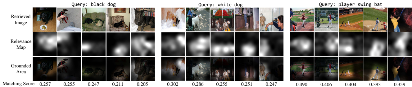
Figure 6. The relevance maps and grounded areas obtained from the retrieved images w.r.t. three queries. The temperature of the softmax for visualizing the relevance map is \tau = 0.1 . Pixels in white indicates a higher matching score. Note that the third image of the query “black dog” contains two dogs, while our model successfully locates the black one (on the left). It also succeeded in finding the white dog in the first image of “white dog”. Moreover, for the query “player swing bat”, although there are many players in the image, our model only attend to the man swinging the bat.
