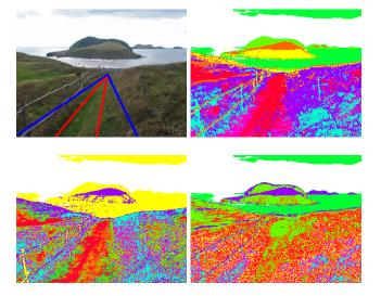
Fig. 3. Hypothetical trail triangle region and sample k-means labels for different cues. Clockwise from upper-left: Central trail region (red) and neighboring regions (blue); cluster labels using **LAB** features (k = 8); labels using **L** features; and labels using **AB** features. For this image, a maximum appearance likelihood of 0.693 was found with **AB** (the maximum for **LAB** is 0.655; for **L** it is 0.523).
