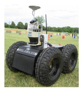
Fig. 2. "Warthog": Segway RMP 400 robot platform with color camera, SICK ladar, and sagitally-mounted Hokuyo URG
