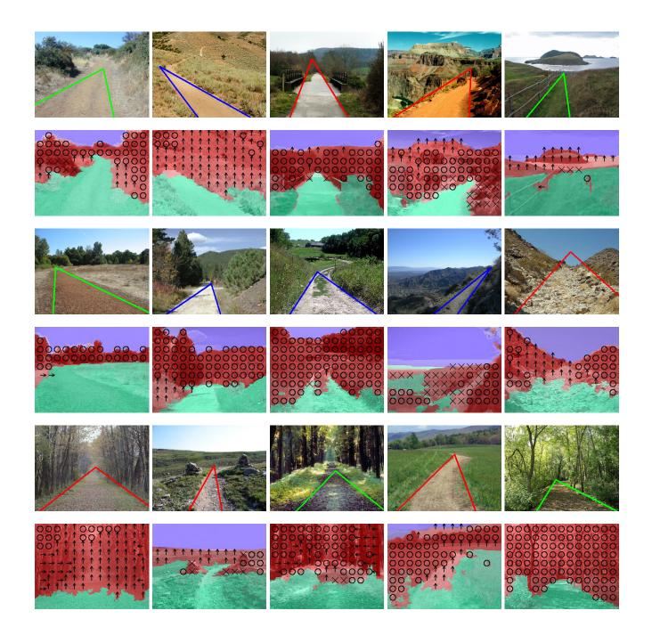
Fig. 6. Results on single-image trail triangle finder on subset of the Web trail data set (see text). Odd rows are output of vision-only component of this paper's algorithm; even rows are output of [38]. Colors indicate which features were automatically chosen as most discriminative: red for LAB, green for AB, and blue for L.
