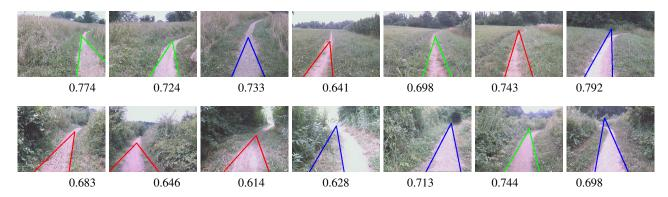
Fig. 8. Results of trail triangle tracker on long hiking trail sequence, shown at 1000-frame intervals. Colors indicate which features were automatically chosen as most discriminative, numbers are overlap with ground truth on that frame. The mis-segmentation in the middle of the bottom row could be eliminated with hysteresis of the trail color.
