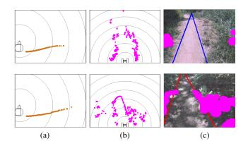
Fig. 5. Filtering ladar groundstrike, two examples. (a) Sideview of robot platform showing sagittal ground profile from Hokuyo data; (b) Overhead view of simultaneous SICK ladar scan; (c) Camera view of trail with SICK ladar points projected (groundstrikes removed). The groundstrike distance was calculated as 2.3 m in the first example and 3.1 m in the second.
