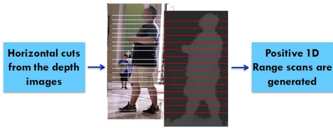
Fig. 3. 1D range scans are generated from the depth camera data for each positive window.
