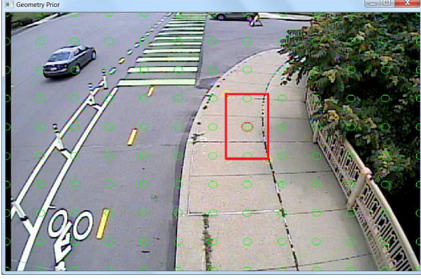
Figure 5: The scale priors of the detection windows for some points are obtained from the user with the help of a software. These points are uniformly distributed in the image. The user provides the expected scale info for each green colored point in the image.
