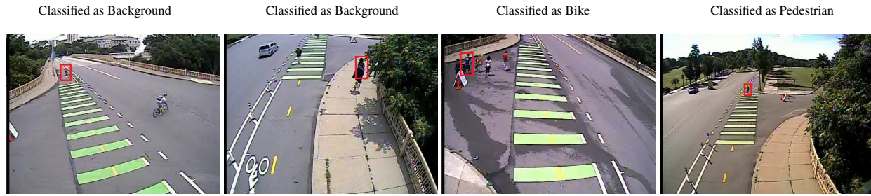
Figure 7: Some false detections of the cascaded detector. Column headings show the classification results of the detector. Low resolution of far objects, and/or partial occlusion are main reasons of the failure cases.
