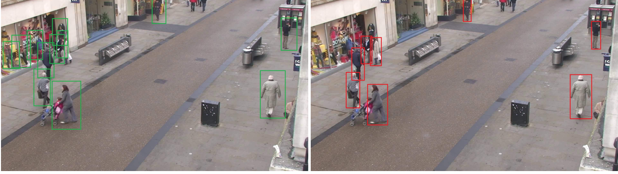
Figure 6: Sample results of the raw and extended detectors from TownCentre dataset. First column displays the output of the raw detector. Second column shows the results of the extended detector. Proposed detector produces better fitted detection windows in addition to eliminating some false alarms.
