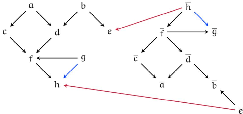
$$(\bar{a} \vee c) \wedge (\bar{a} \vee d) \wedge (\bar{b} \vee d) \wedge (\bar{b} \vee e) \wedge \\ (\bar{c} \vee f) \wedge (\bar{d} \vee f) \wedge (\bar{g} \vee f) \wedge (\bar{f} \vee h) \wedge (e \vee h)$$
