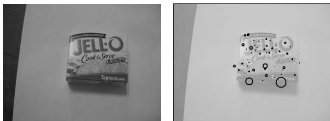
Fig. 3. A snapshot from the training sequence of the kitchen domain (left) and the locations of its annotation-filtered PCA-SIFT keypoints (right).
