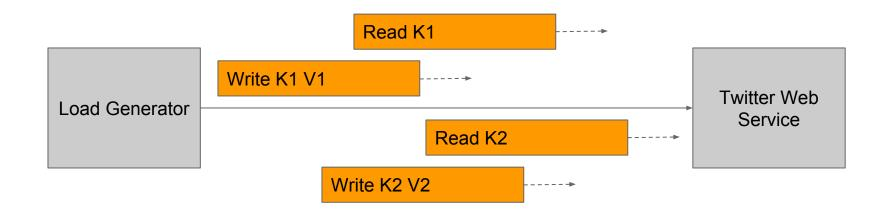
Network delay causes a read to happen before a write, which was not expected by the grader
