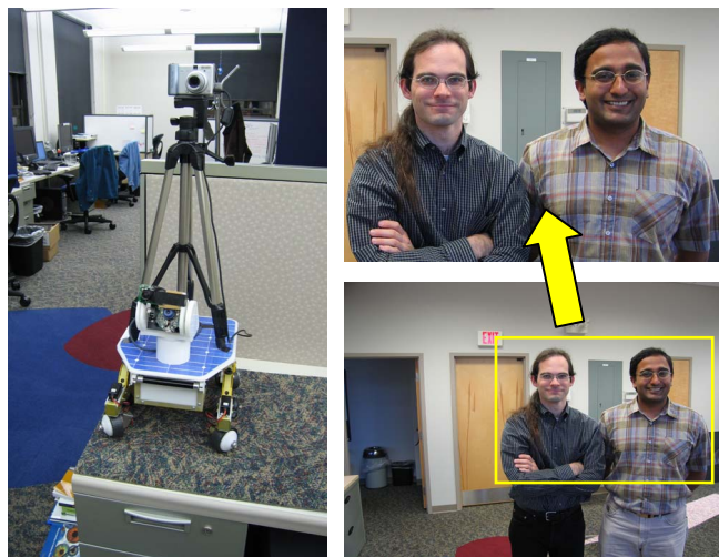
Fig. 1: The Robot Photographer, and an Example of Picture-Framing The cropped, resized image at the upper right is automatically produced by the algorithm described in this paper. The original source image is shown at the lower right
