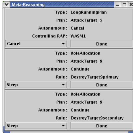
Fig. 3. A view of the interface the human uses to make decisions. Three decisions are shown. At the top is a decision whether to cancel a long running plan. Below are two unallocated roles from the same plan, for destroying a particular target.
