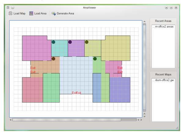
Figure 11: Areas detected (after outside-removal, inaccessible area culling, and merging) in *medium-office2.gw*. Note that the two green areas on the right side are distinct, though their shading is similar.
