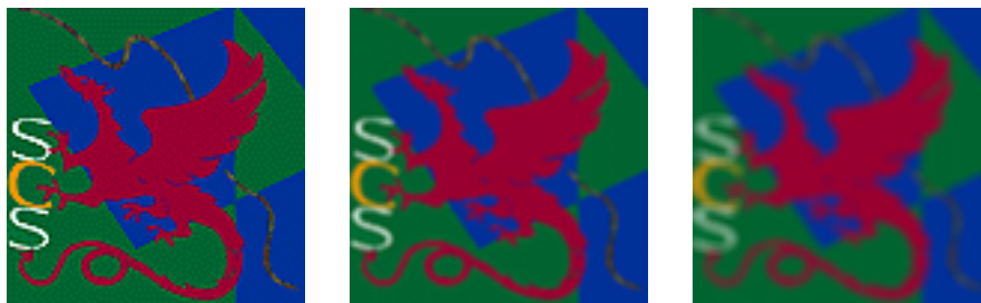
Figure 5: The SCS Dragon: original image (left), blurred slightly with a 3 \times 3 mask (middle), and blurred with a 5 \times 5 mask (right). See text for mask values.
