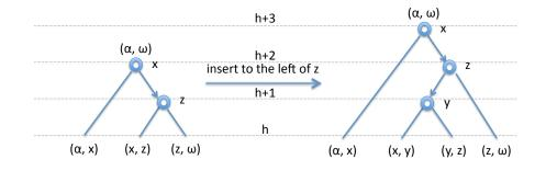
In the situation on the right, the subtrees labeled  $(\alpha, x)$  and  $(z, \omega)$  must have exactly height *h*, but only one of (x, y) and (y, z). In this case, a single left rotation alone will not restore the invariant (see Exercise 1). Instead, we apply a so-called *double rotation*: first a *right* rotation at *z*, then a *left* rotation at the root labeled *x*. When we do this we obtain the picture on the right,
