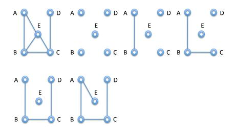
The first graph is the given graph, the completely disconnected graph is the starting point for this algorithm. At the bottom right we have computed the spanning tree, which we know because we have added n - 1 = 4 edges. If we tried to continue, the next edge *BE* could not be added because it does not connect two trees, and neither can *CE*. The spanning tree is complete.
