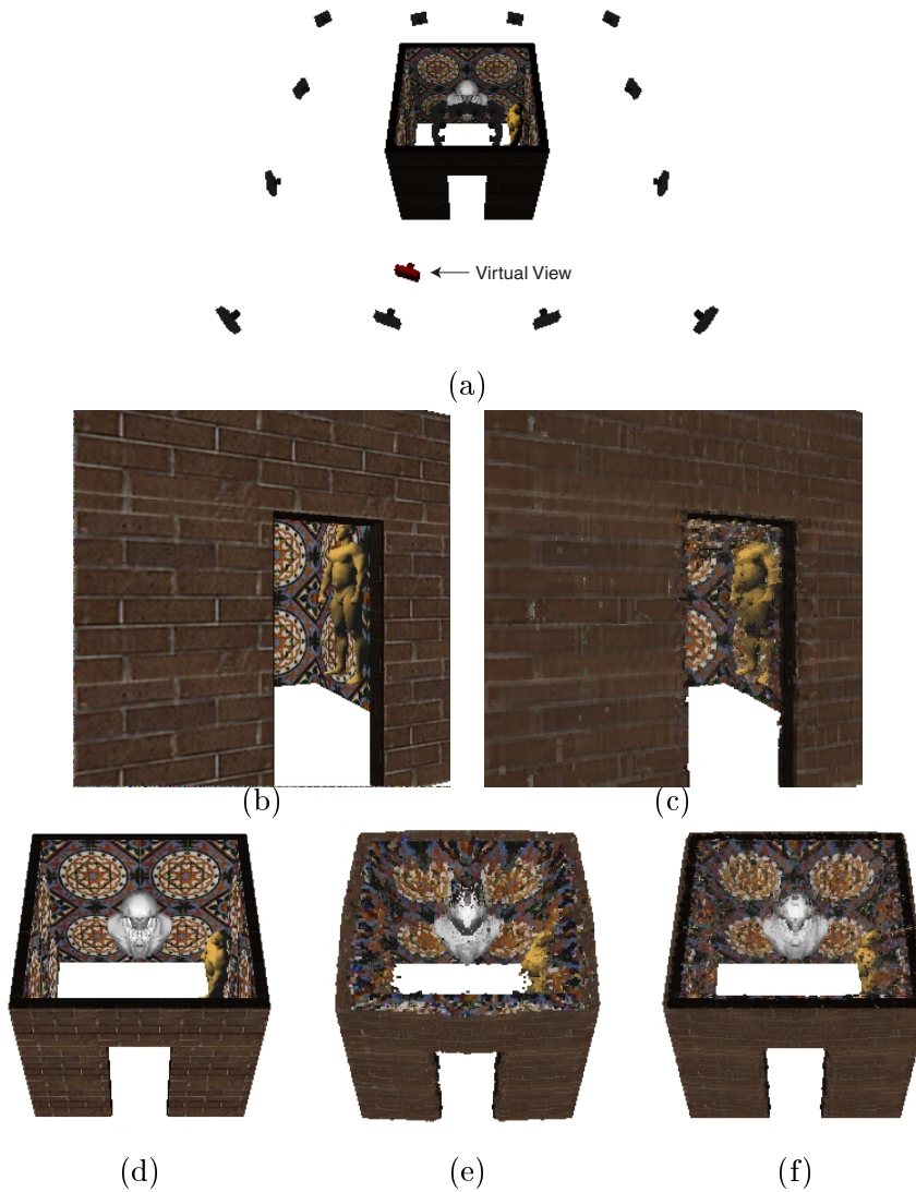
Figure 11. Reconstruction of a synthetic building scene. (a) 24 Cameras were placed in both the interior and exterior of a building to enable simultaneous, complete reconstruction of its exterior and interior surfaces. The reconstruction contains 370,000 voxels, carved out of a 200 \times 170 \times 200 voxel block. (b) A rendered image of the building for a viewpoint near the input cameras (shown as “virtual view” in (a)) is compared to the view of the reconstruction (c). (d-f) Views of the reconstruction from far away camera viewpoints. (d) shows a rendered top view of the original building, (e) the same view of the reconstruction, and (f) a new reconstruction resulting from adding image (d) to the set of input views. Note that adding just a single top view dramatically improves the quality of the reconstruction.
