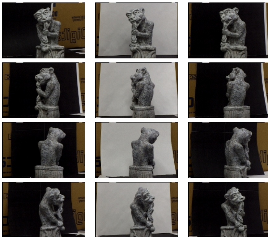
Figure 7. Nine of sixteen 486x720 RGB images of a gargoyle stone sculpture. The sequence corresponds to a complete circumnavigation of the object, performed in approximately 22.5 degree increments.
