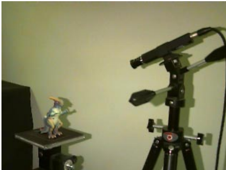
Figure 8: Image Acquisition Setup. Basis images were captured by placing an object on a calibrated pan-tilt head and rotating the object in front of a stationary video camera. The camera was placed above the object to satisfy the ordinal visibility constraint.
