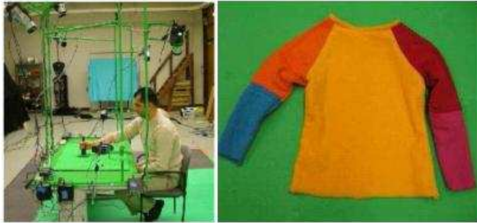
Figure 2.1: The experimental setup. At left is a desktop instrumented with cameras and at the right is a colorful jersey used to facilitate tracking.
