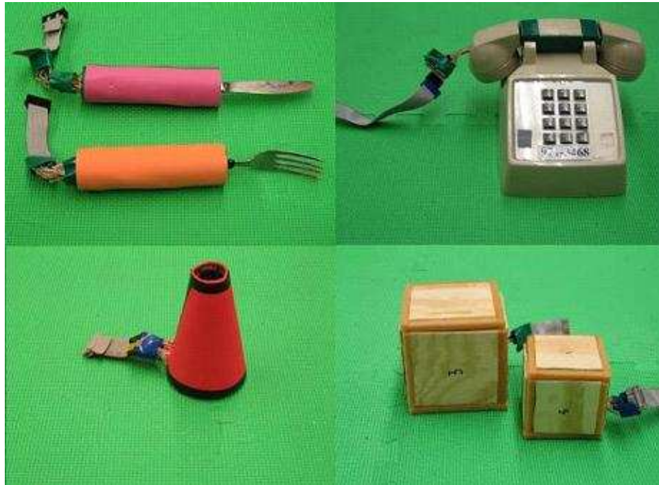
Figure 2.3: A selection of force sensing objects. These include a force sensing phone, a cube and eating utensils.
