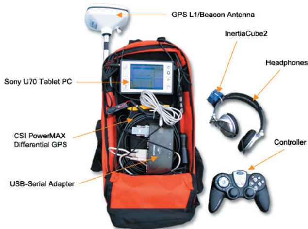
Figure 3: The equipment carried by the user in “The Voices of Oakland.” The wizard wears headphones and uses a Tablet PC that communicates wirelessly with the user’s tablet.
