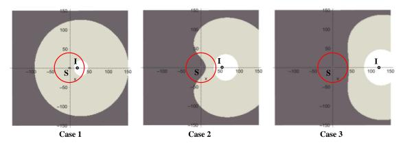
For this problem, assume frames will be received in the dark shaded areas and will be lost in the light shaded areas. Assume both S and I are persistently backlogged (always have packets to send). Suppose the physical data rate on the is R.
