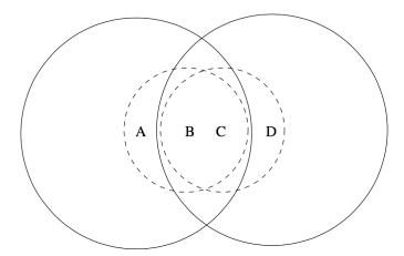
The solid circles represent the transmission radius of nodes A and D, respectively, and the dashed circles represent the transmission range of B and C, respectively. Assume that if two nodes' transmissions will interfere at a location if and only if they transmit at the same time and their transmission areas overlap. In these problems, assume that losses only occur due to collisions.
