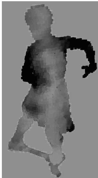
Figure 4.8: The shape intensity coded with the magnitude of the scene flow. Darker pixels are those with larger scene flow values. The motion on the right arm is mostly due to rotation about the torso, and that on the left arm is mostly because of shoulder and elbow movement.
